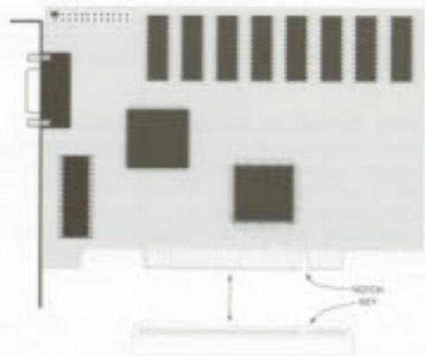
Figure 2-9. Installing a PCI Local Bus Card
